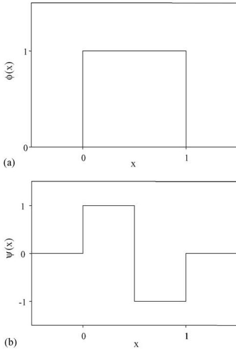
Fig. 2. Orthonormal scaling function and wavelet function of Haar wavelet.
