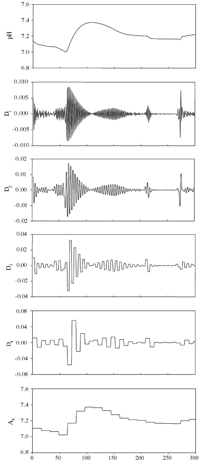
Fig. 3. Multi-resolution plot of pH (decomposition level: 4).
