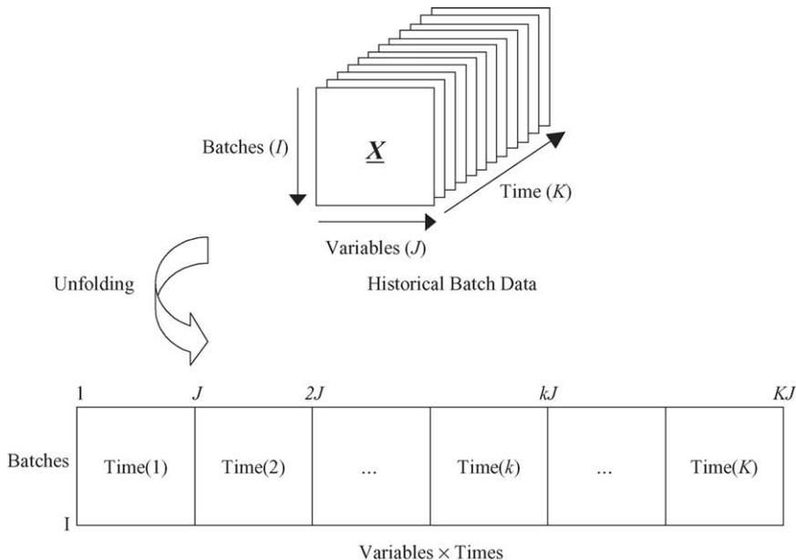
Fig. 1. Decomposition of a three-way data matrix  $\underline{X}$  by MPCA.
