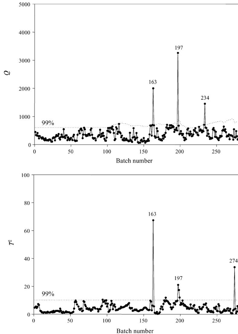
Fig. 8. Adaptive MPCA.  $Q$  and  $T^2$  monitoring charts with 99% confidence limits.
