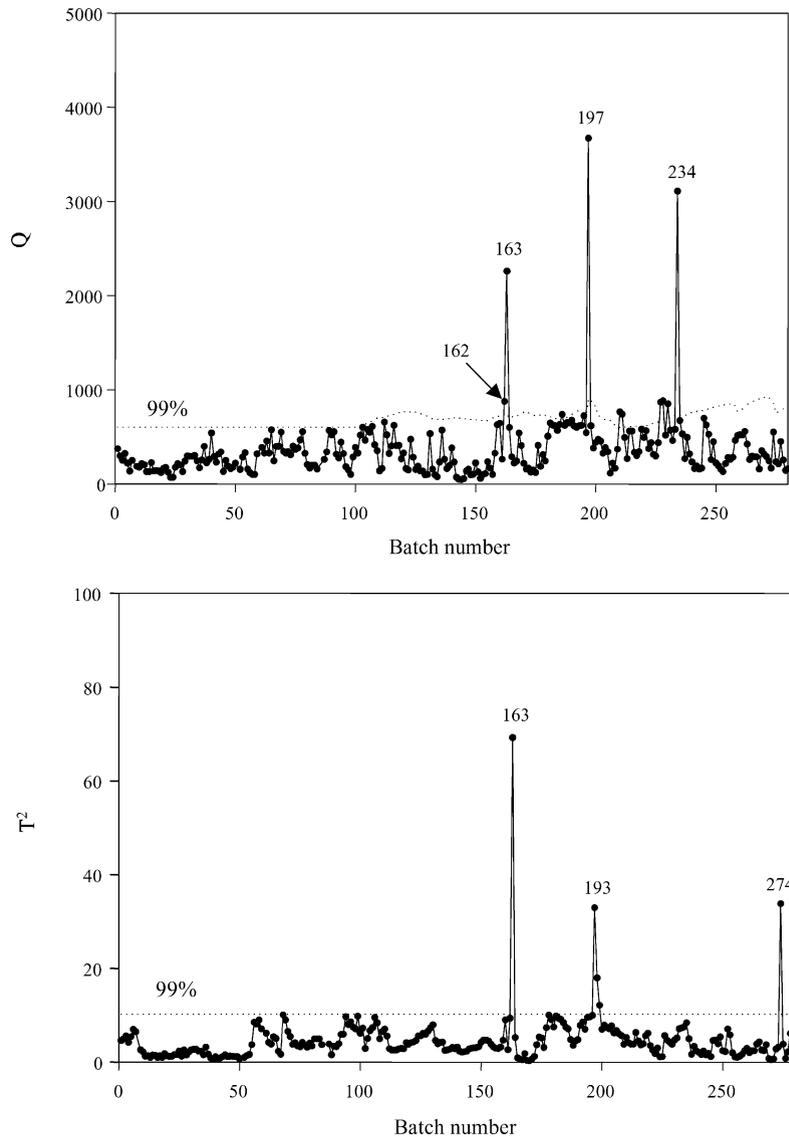
Fig. 9. Unifying adaptive multiscale MPCA.  $Q$  and  $T^2$  monitoring charts with 99% confidence limits.
