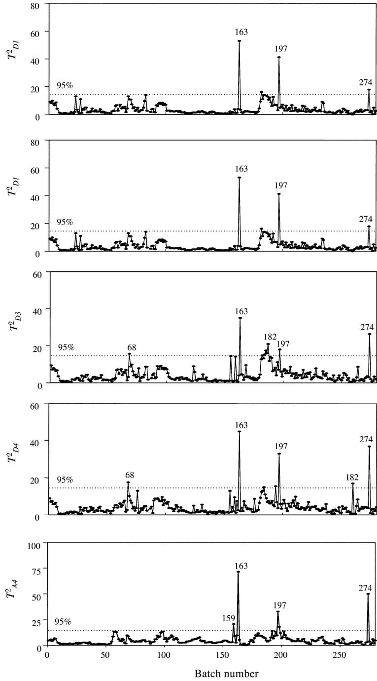
Fig. 11.  $T^2$  monitoring charts at each scale.
