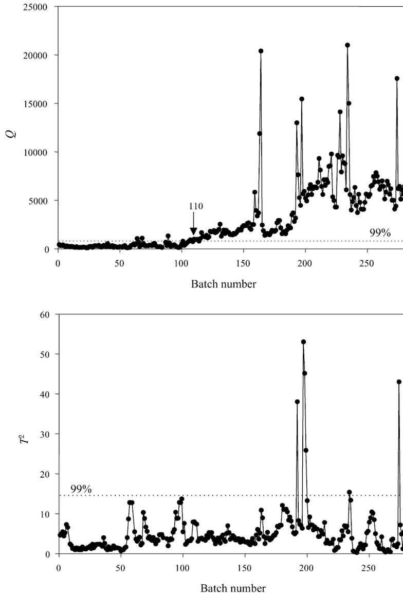
Fig. 7. MPCA.  $Q$  and  $T^2$  monitoring charts with 99% confidence limits.
