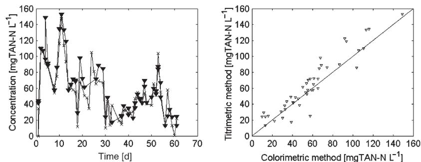
**Figure 5** Comparison between colorimetric and titrimetric measurements for TAN concentrations in the SHARON reactor (left) and corresponding q-q plot (right)
