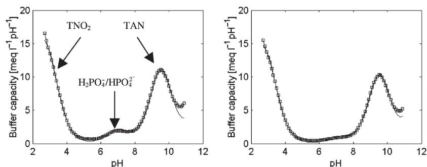
**Figure 4** Typical buffer capacity curves for the period with  $228 \text{ mgPO}_4^{3-}\text{-PL}^{-1}$  phosphate in the influent (left) and the period with  $11 \text{ mgPO}_4^{3-}\text{-PL}^{-1}$  phosphate in the influent (right)
