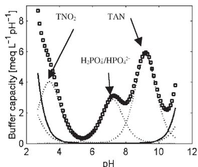
**Figure 1** Contribution of individual components (...) (in casu  $\text{TNO}_2$ , phosphate and TAN) and the water buffer (—) to the buffer capacity curve (□).
