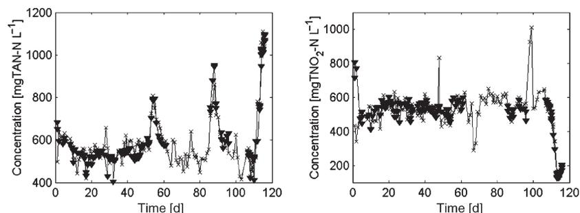
**Figure 2** Top: Comparison between colorimetric (x) and titrimetric measurements (▼) for TAN concentrations (left) and TNO<sub>2</sub> (right) in the SHARON reactor
