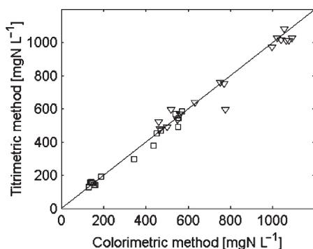
**Figure 3** The q-q plot of TAN (▽) and TNO<sub>2</sub> (◻) for comparing concentration measured in the 17 samples with the colorimetric and titrimetric method
