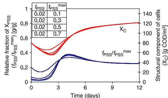
**Figure 4** | Sensitivity of the model during the start-up of a continuous-flow stirred reactor (HRT = 6.5 days).
