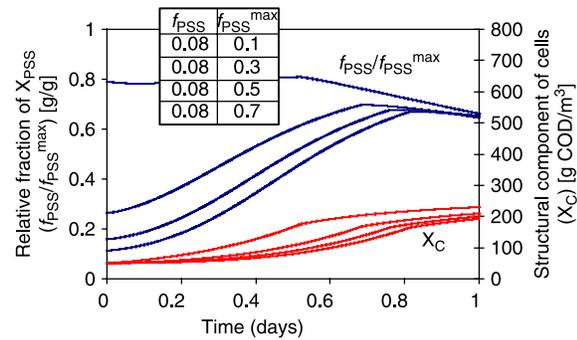
**Figure 3** | Batch reactor.  $S_0/X_0 = 10$ . Sensitivity analysis for initial values of  $f_{PSS}/f_{PSS}^{\max} = 0.8; 0.27; 0.16; 0.11$  units/g.
