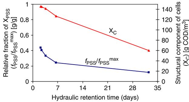
**Figure 5** | Semi-continuous-flow stirred reactor. Sensitivity of the model to hydraulic retention time ( $f_{PSS}^{max} = 0.5$  units/g).
