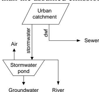
**Figure 2.** Addition of storm water infiltration ponds to the previously modelled setup
