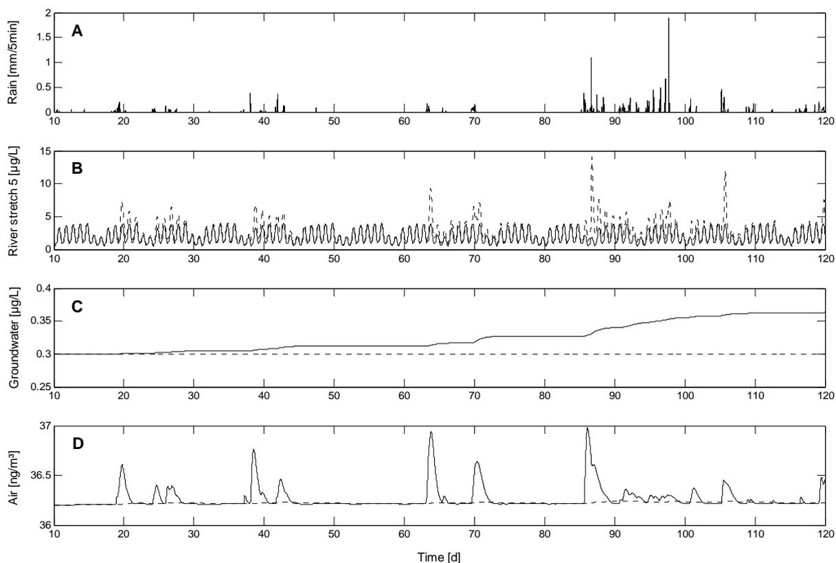
**Figure 3.** Input rainfall series (A) and simulated DEHP concentration in the two modelled scenarios (basic scenario in dotted line, scenario with the stormwater infiltration ponds in solid line) in the last river stretch of the IUWS model (B), in the groundwater compartment of the MFTM (C) and in the air compartment of the MFTM (D)
