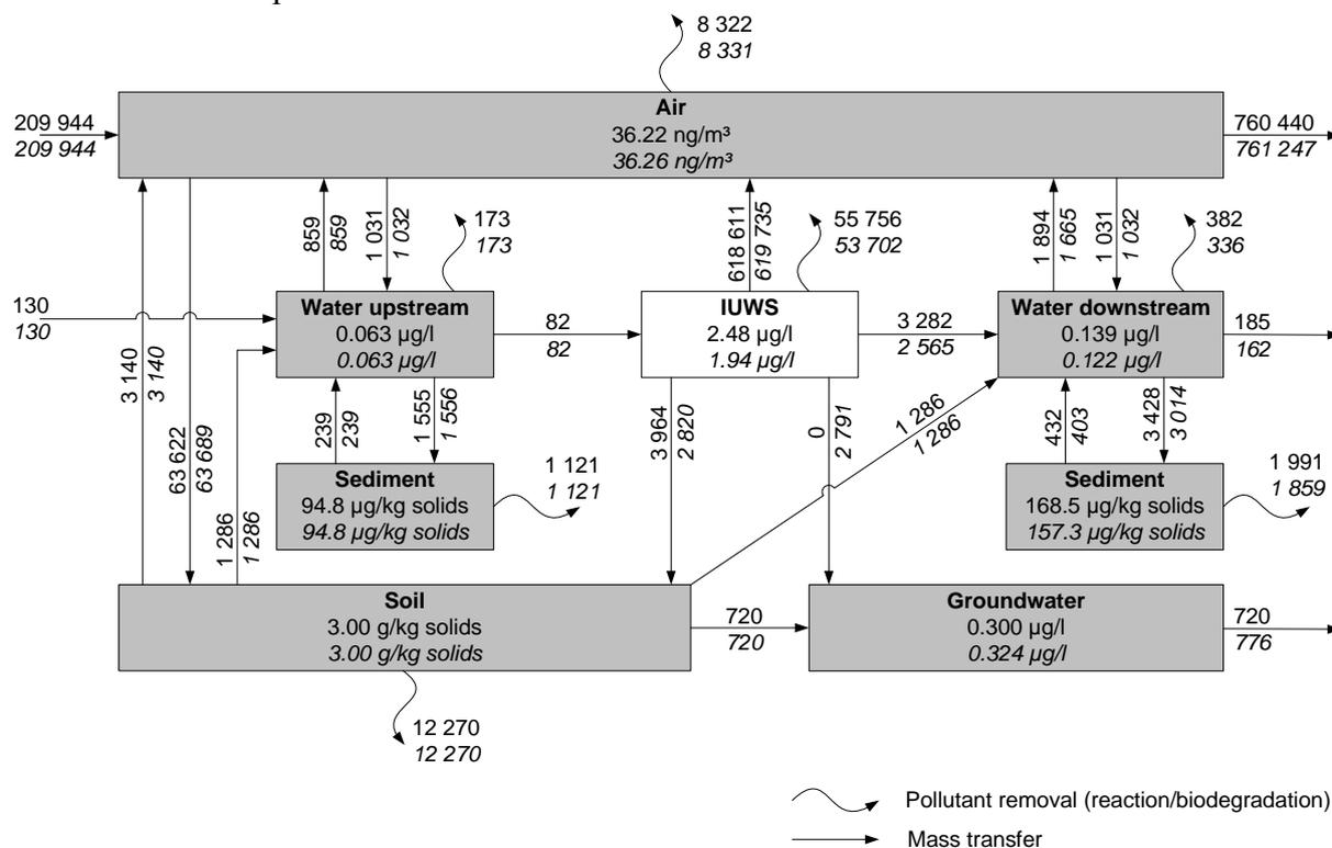
**Figure 4.** Mean DEHP mass fluxes (in  $\text{g}\cdot\text{d}^{-1}$ ) and concentrations in the modelled system: reference scenario (normal typeface) and after the implementation of stormwater infiltration ponds (italic typeface); values in the IUWS block are concentrations in the receiving water after mixing, i.e. at the outflow of river stretch 5.
