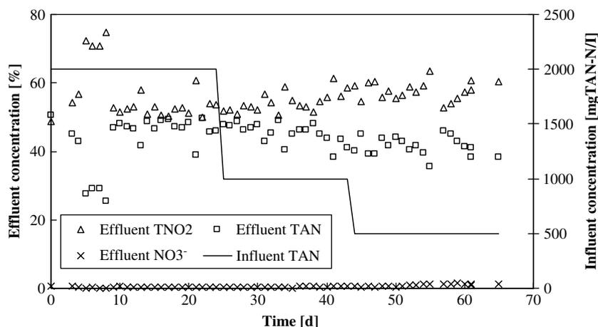
**Figure 1.** Lab-scale SHARON influent TAN concentration (—) and effluent TAN (□), TNO<sub>2</sub> (Δ) and nitrate (x) concentration during the experimental period.
