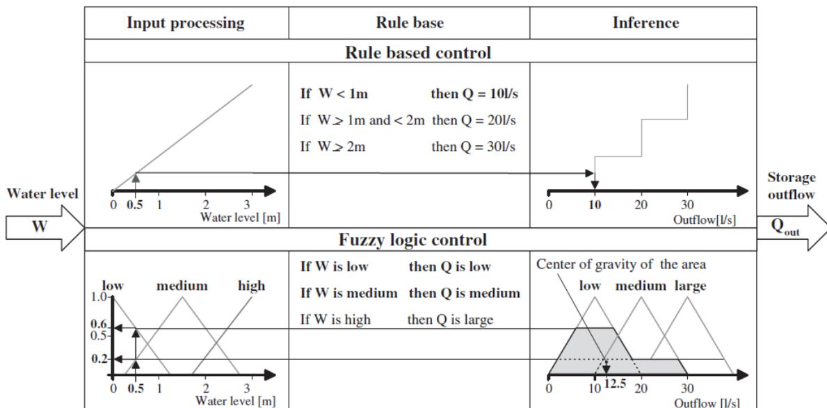
**Figure 3.** Fuzzy Logic Control (source: Klepiszewski and Schmitt, 2002)
