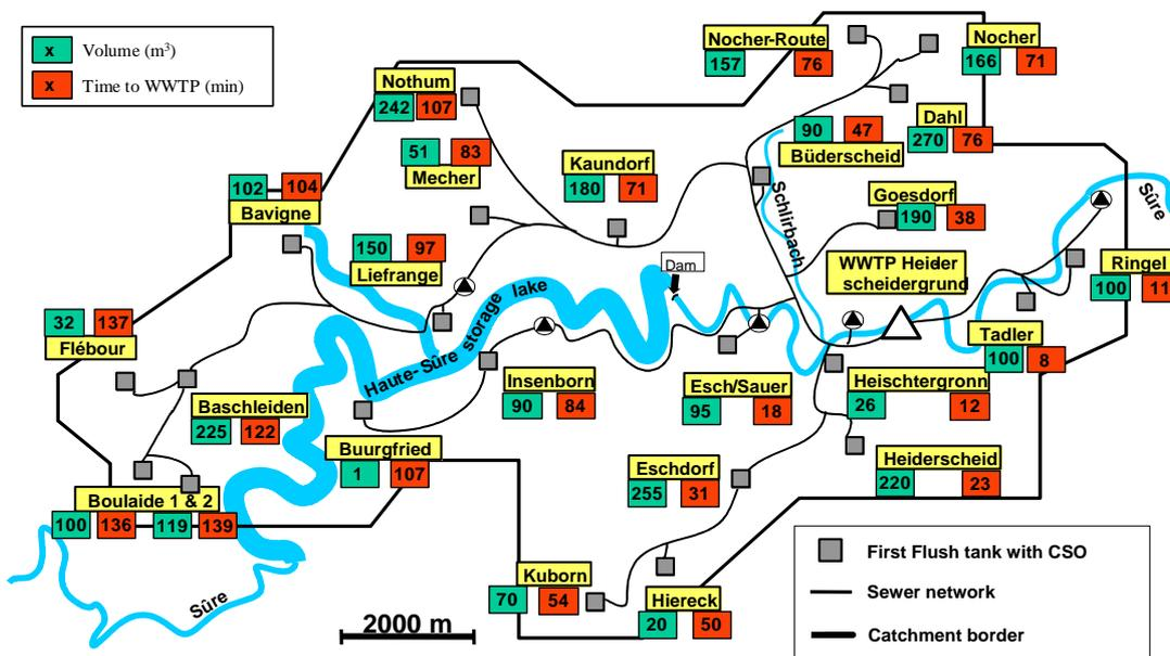
**Figure 5.** The ultimate Haute-Sûre wastewater system
